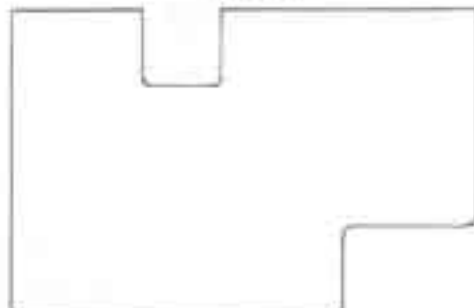
All internal cut outs should have radius corners.
